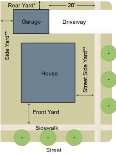
Figure 1: Corner Lot - Detached Garage
